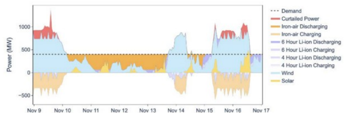
Exhibit 57: Long Duration Energy Storage such as iron-air batteries can help to stabilise the grid to meet periods of low wind & sun resource
